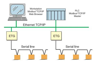
**Remote device diagnostic** — A web page on the gateway allows monitoring of memory areas on the serial devices for quick maintenance or verification of communications health.
