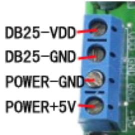
JN1&JN2 connected , is the case of the single power , the POWER + and the isolating source will be connected, the GND and the isolating source GND will be connected: if the JN1&JN2 is open circuit , the POWER + and the isolating source will be cut off, the GND and the isolating source
