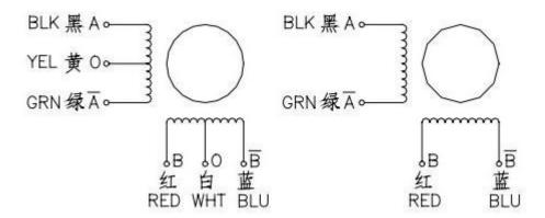
There are two ways to wire, the front one is high turning speed, and the later one is high holding torque.
