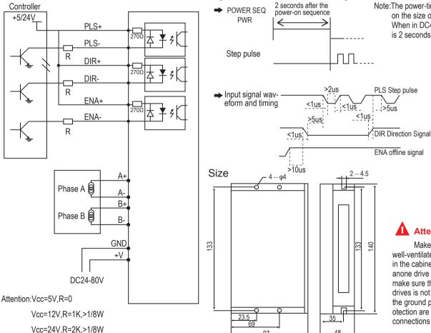
Note: The power-time of the drive depends on the size of the Plus AC voltage, When in DC48V Typical power-time is 2 seconds
