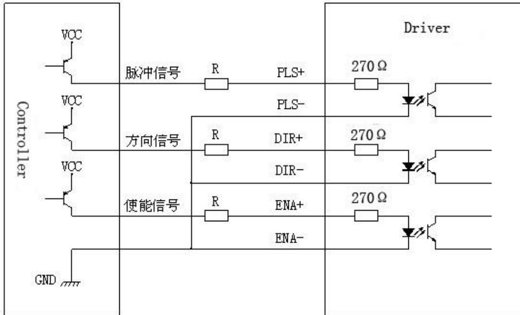
Fig. 2 Input port circuit ( Yin connection)
