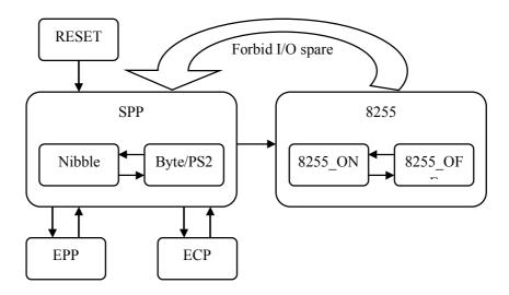
In SPP mode, use software to control PCR and query PSR to realize Nibble, Byte and PS/2 etc. transfer, the detail information can consult IEEE1284 criterion.
