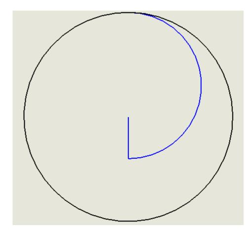
Hyperherm ramps the kerf to get sort of like a spiral in some cases, TD does it with a line/arc/J and Kjellberg uses a J:
