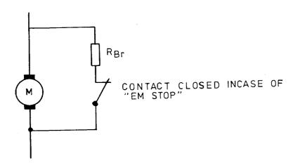
For short circuiting the motor you can use a normally closed contact of a normal auxiliary contactor (e.g. Siemens 3TA66) or the auxiliary contact (normally closed contact) of a power contactor.
