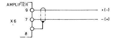
Caution: For command values related to earth with only one command value line this must be connected to terminal 9.
