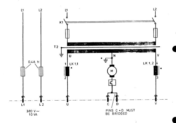
CAUTION: OBSERVE THE CHOKE POLARITY! FOR AUTOTRANSFORMERS DO NOT GROUND THE CENTRE POINT (N).
