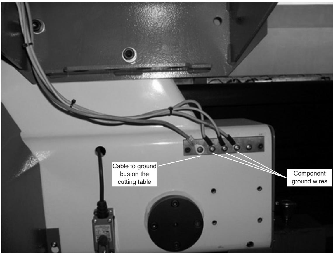
Example of a good gantry ground bus. It is bolted to the gantry, close to the motor. All of the individual ground wires from the components mounted on the gantry go to the bus except those from the RHF module and the torch holder. A single heavy cable then goes from the gantry ground bus to the ground bus bolted to the table.
