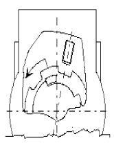
Locked turret (rollers at the beginning of the cam top face (313 proximity operating)
