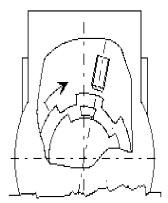
The pictures represent the stages corresponding to the toolholder disc clockwise rotation; for the counterclockwise rotation, movements are reversed.
