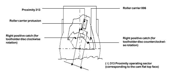
Released turret (the rollers are at the bottom of the cams - the Hirth coupling are released)
