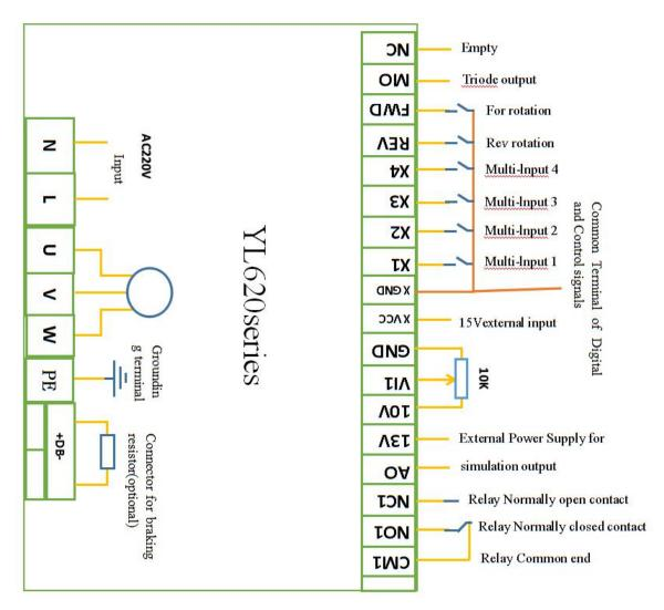
Note: The above wiring diagram explained that only supplies the reference, take the actual product as the standard. The diagram is subject to change without notice.
