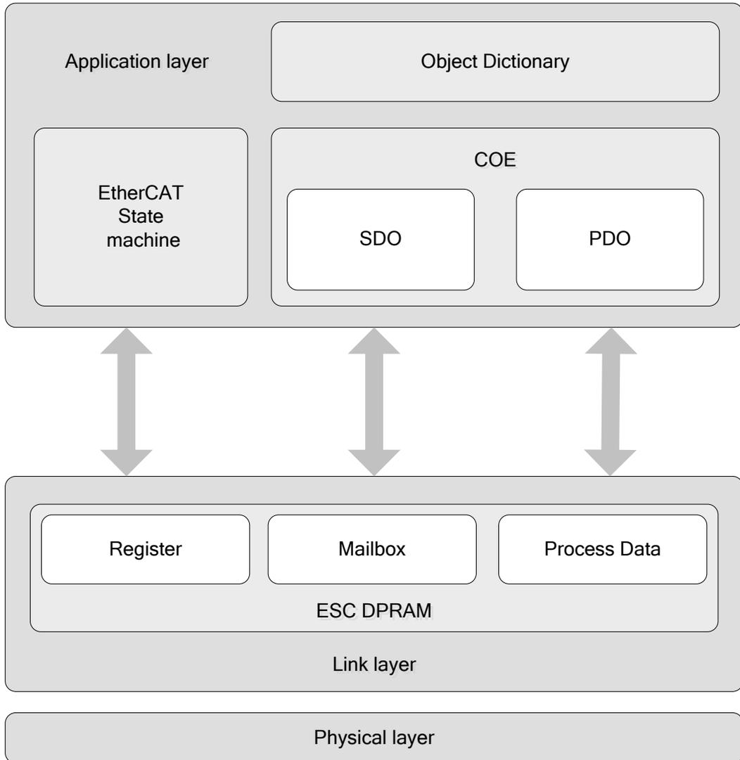
Figure3-1 Communication structure
