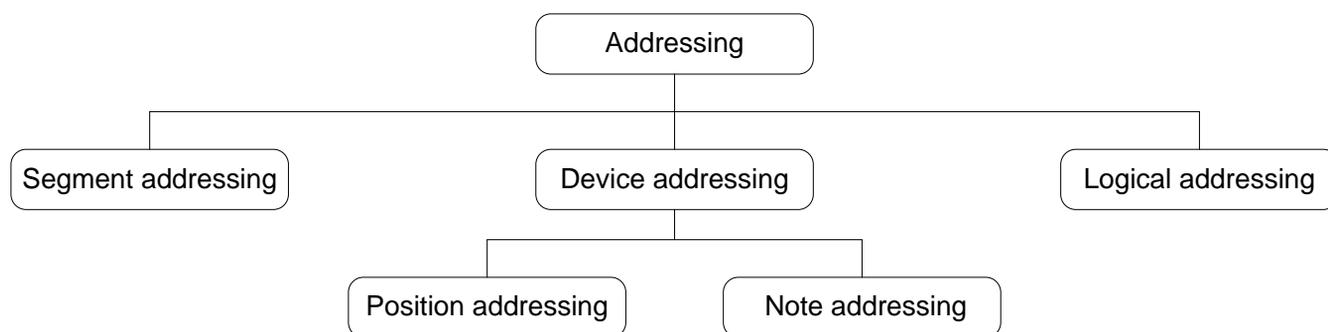
Device addressing for EtherCAT includes location addressing and node addressing. The location addressing is assigned by the master station according to the connection order of the slave devices. The node addressing can be assigned by the master station as needed or by the slave station by parameter assignment of the node address, and the master station then looks for a particular node by the node address.
