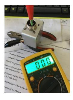
Pin 3 = 0 ohms, closed circuit.
