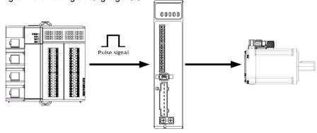
Pulse-controlled versions of servo motors can rotate in both directions. This means a controller needs to provide, at a minimum, two control signals to the drive. There are two ways to provide these signals: "Step/Direction mode" or "CW/CCW mode" or "clockwise/counterclockwise mode". Both modes require two control signals from the controller to the drive. Max. frequency for both input mode signal is 500kHz(Differential), 300kHz(Single-ended).
