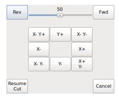
This is a dialog which allows the torch to move away from the cut to find a good piece of material to restart the cut from. This function is only available from the Extras panel and is only valid while paused.
