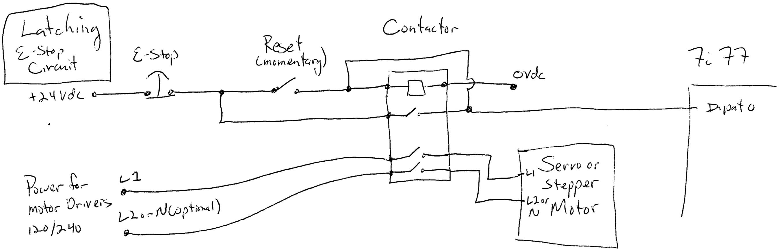
Inputs & Outputs Wired to 7c77
